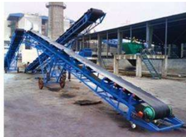
WASTE SAND CONVEYOR WITH MAGNETIC SEPARATOR
