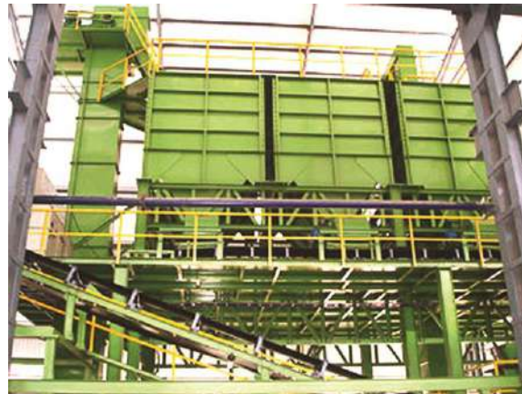
Sand hoppers : 500 kg to 100 ton & Bucket elevators
